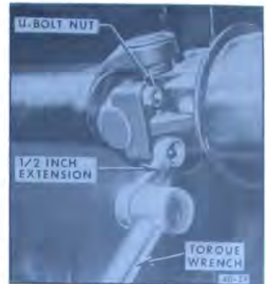
Figure 40-53—Using Extension to Torque U-Bolt Nuts
