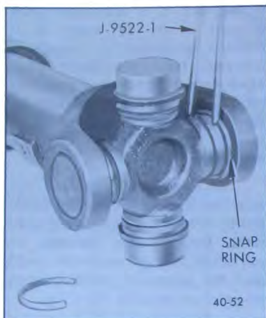
Figure 40-46—Removing Snap Rings from Propeller Shaft
