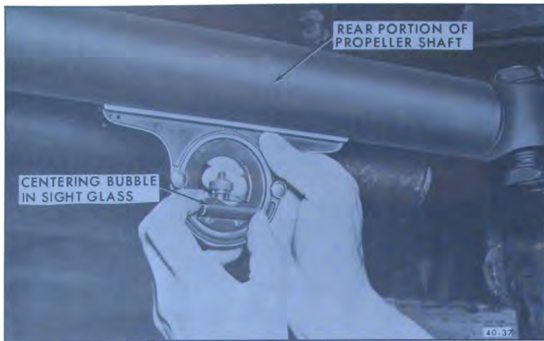
Figure 40-59—Measuring Angle at Rear of Propeller Shaft
