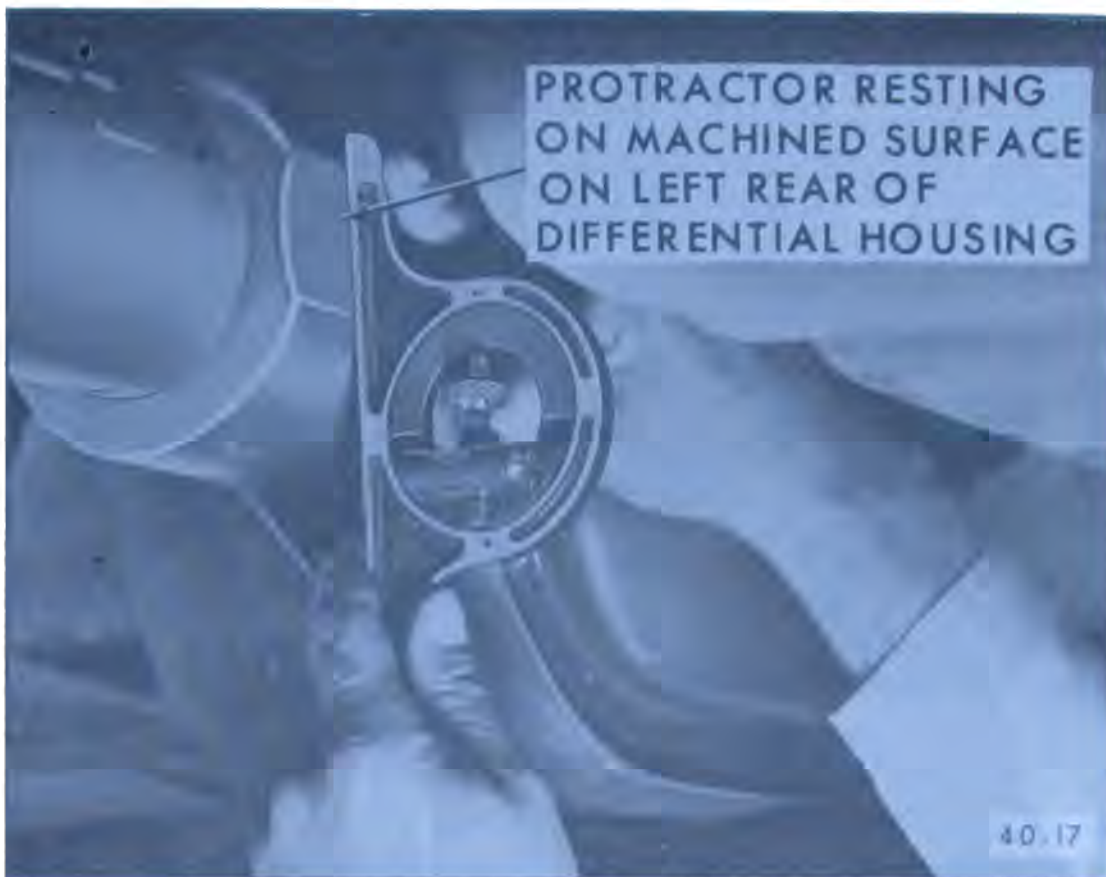
Figure 40-58—Measuring Differential Assembly Angle
