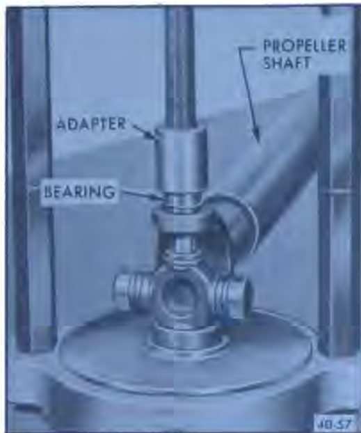
Figure 40-51—Pressing Bearing into Place
