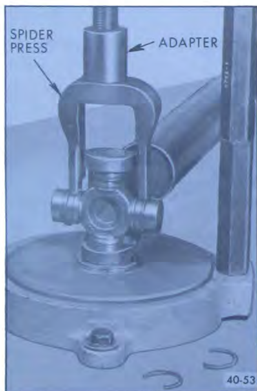
Figure 40-47—Pressing Out U-Joint Bearings
