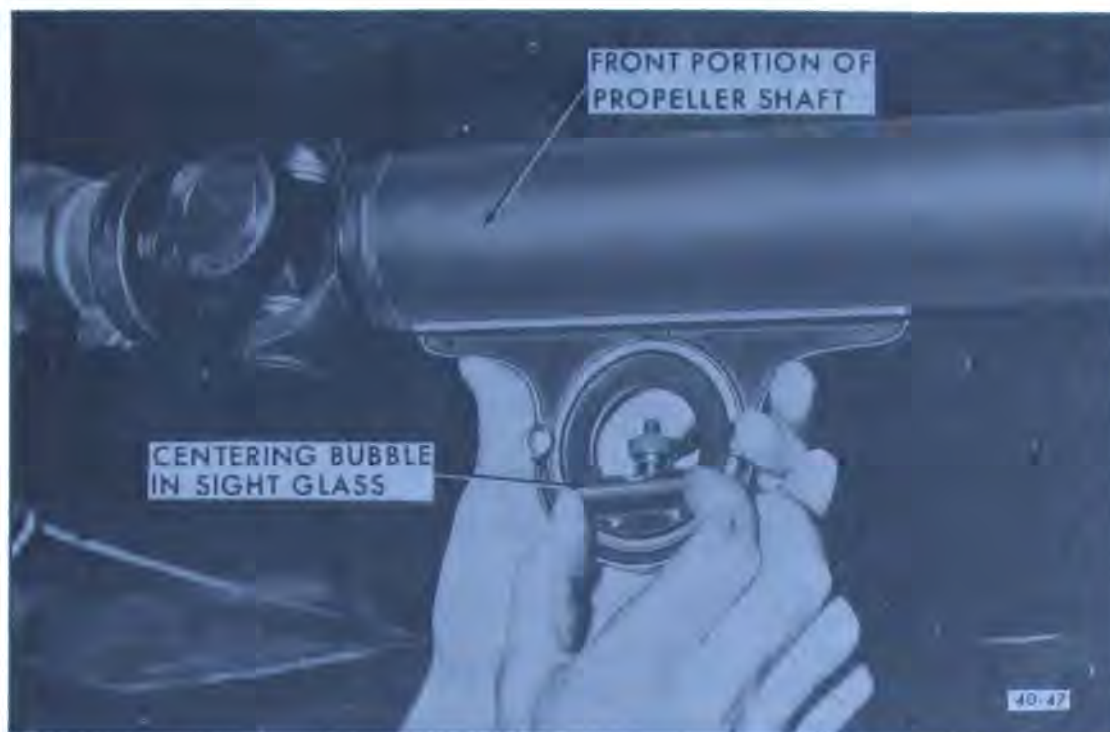
Figure 40-61—Measuring Angle at Front of Propeller Shaft
