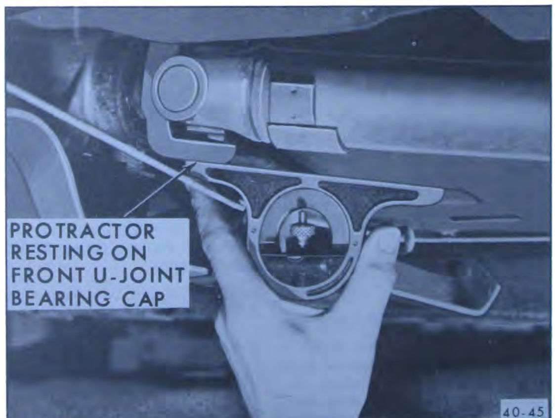
Figure 40-60—Measuring Transmission Angle
