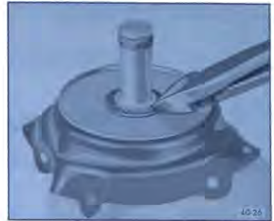
Figure 40-32—Removing Diaphragm Retainer
