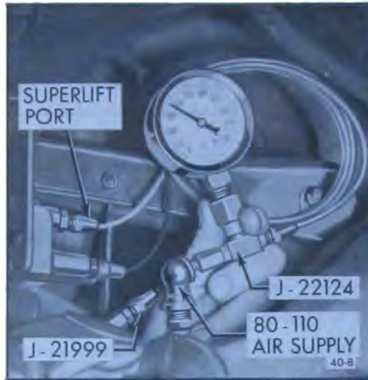
Figure 40-9—Connect Test Gage to Superlift Outlet
