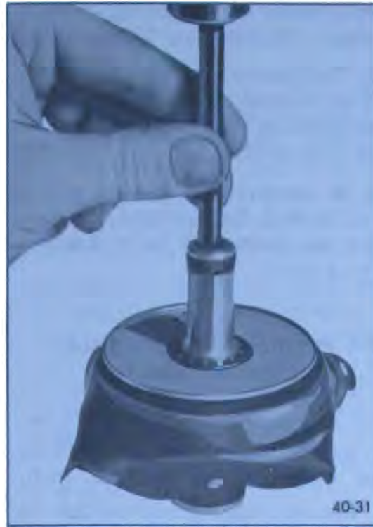
Figure 40-36—Installing Check Valve
