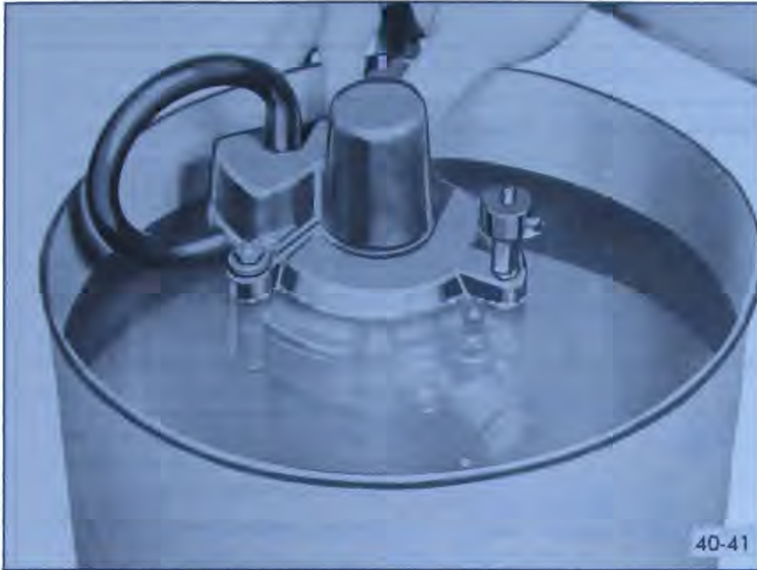
Figure 40-44—Checking Compressor, Reservoir Tank and Regulator for Leaks
