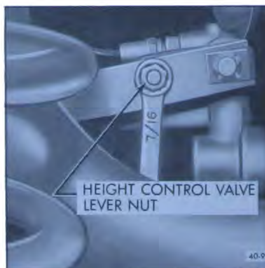
Figure 40-10—Loosen Height Control Valve Lever Nut
