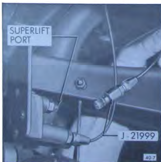
Figure 40-8—Remove Superlift Air Supply Line
