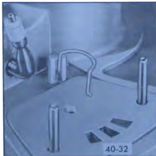
Figure 40-37—Installing Valve Tension Spring in Boss
