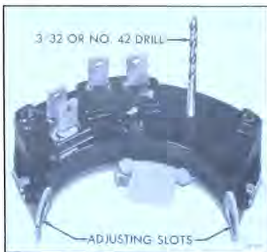
Figure 120-11—Adjusting Neutral Safety Switch
