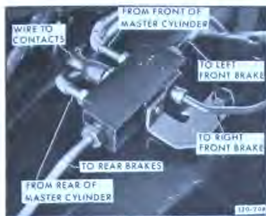
Figure 120-12—Distributor and Brake Failure Warning Switch Assembly
