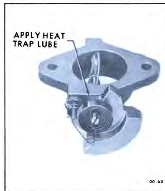
Figure 00-15—Lubricating Points on Manifold Heat Control Valve - 350, 400 and 430 Cu. In. Engines
