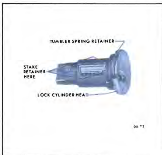
Figure 00-8—Installing Spring Retainer
