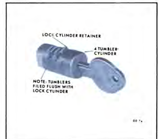
Figure 00-10—Coded Glove Compartment Lock Cylinder
