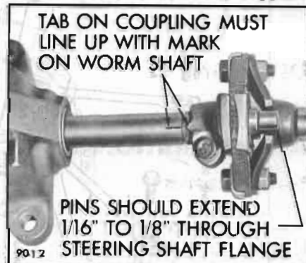
Figure 90-77—Flexible Coupling Installation
