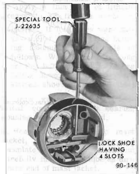
Figure 90-101—Driving Out Release Pin
