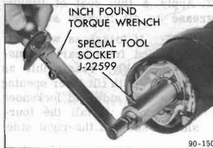
Figure 90-106—Adjusting Steering Shaft Torque
