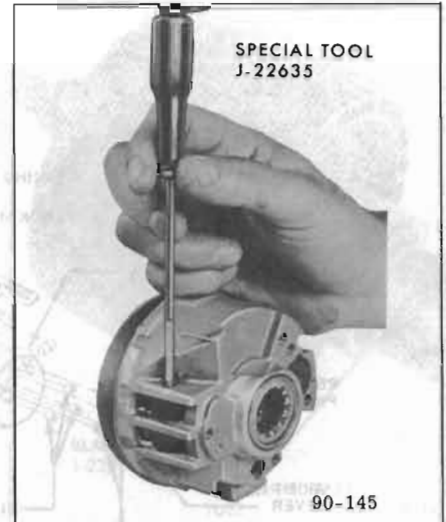
Figure 90-100—Driving Lockshoe Pin Flush with Housing Face
