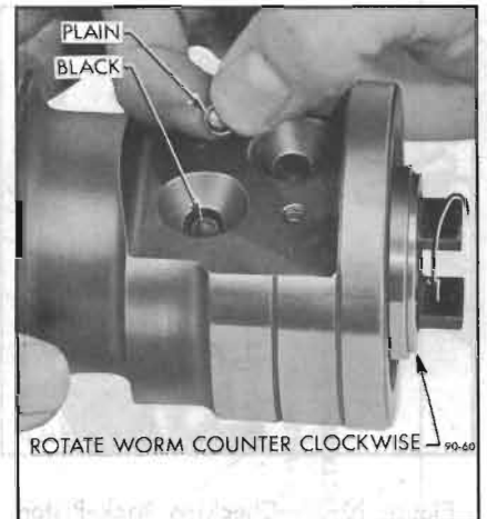
Figure 90-56—Loading Balls in Rack-Piston Nut
