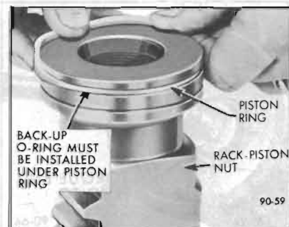
Figure 90-55—Installing Rack-Piston Ring on Rack-Piston Nut
