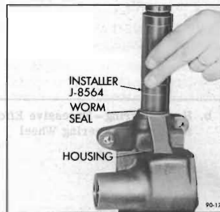
Figure 90-12—Installing Worm Shaft Seal
