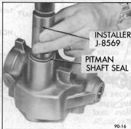
Figure 90-11—Installing Pitman Shaft Seal
