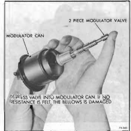
Figure 74-360—Checking Modulator Can Assembly
