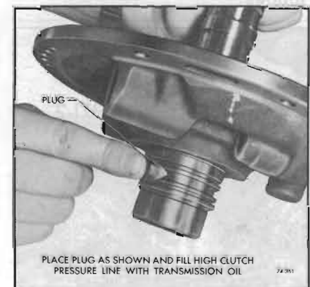
Figure 74-361—Checking Cross Leakage Between Pump Cover and Stator Shaft
