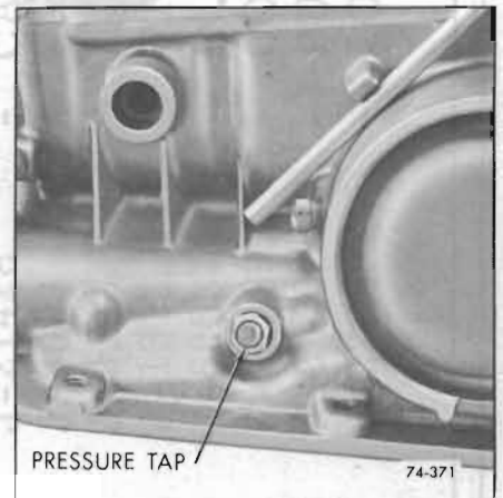
Figure 74-371—Super Turbine "300" Transmission Pressure Checks
