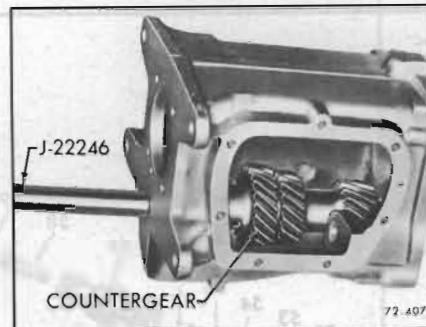
Figure 72-407—Removing Counter Gear
