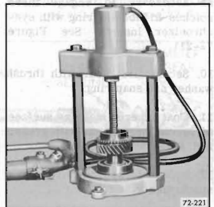
Figure 72-221—Installing Main Drive Gear Bearing
