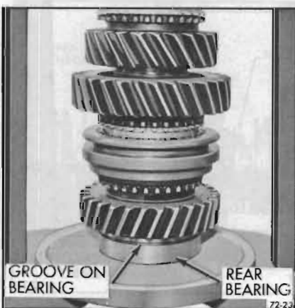
Figure 72-23—Installing Rear Bearing
