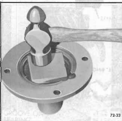
Figure 72-33—Installing Front Bearing Retainer Seal
