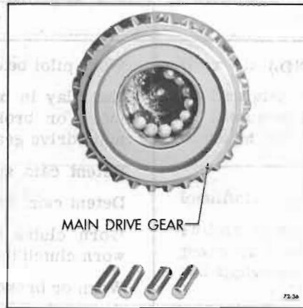
Figure 72-36—Installing Needle Bearings
