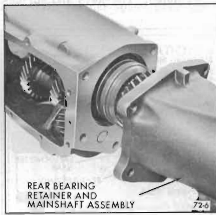
Figure 72-6—Removing Mainshaft Assembly
