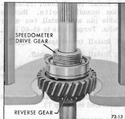
Figure 72-13—Removing Speedometer Drive Gear
