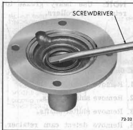
Figure 72-32—Removing Front Bearing Retainer Seal
