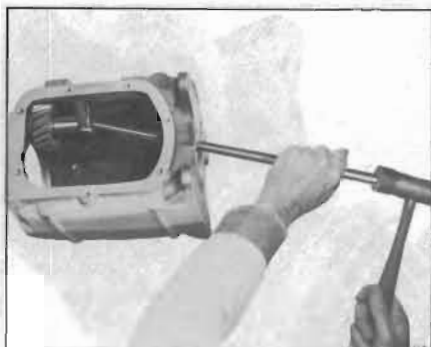
Figure 72-9—Removing Reverse Idler Shaft
