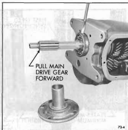
Figure 72-4—Removing Front Main Bearing
