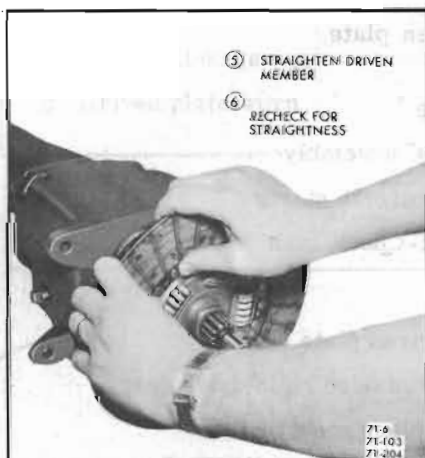
Figure 71-7—Checking Driven Plate Run-out
