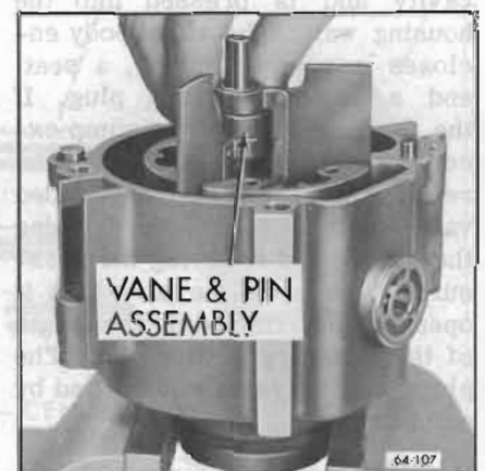
Figure 66-12—Installing Vane and Pin Assembly in Rotor
