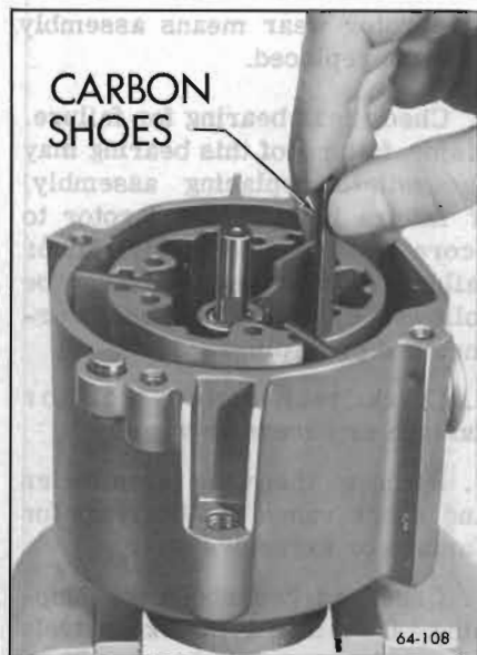
Figure 66-15—Installing Carbon Seal and Rotor Ring
