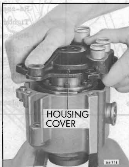
Figure 66-16—Installing Housing Cover
