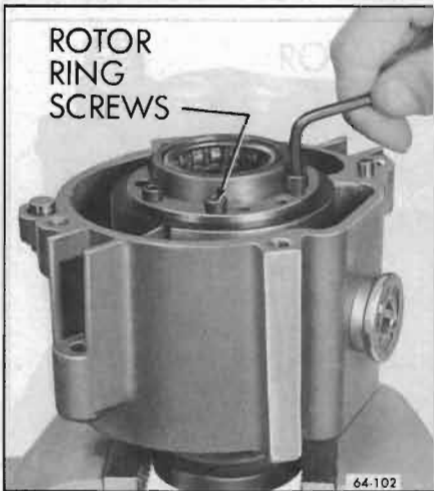
Figure 66-7—Removing Rotor Ring Screws
