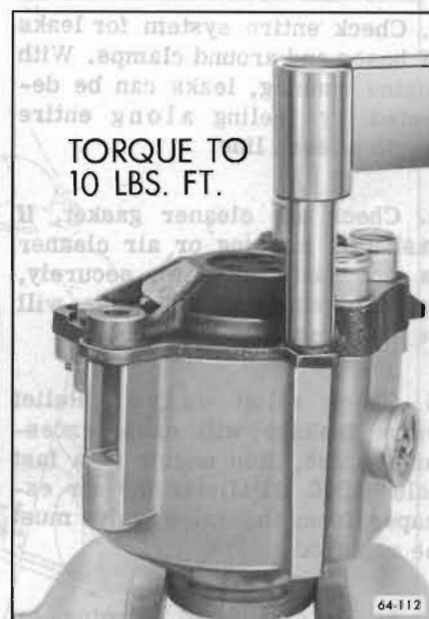
Figure 66-17—Torquing Housing Cover Bolts
