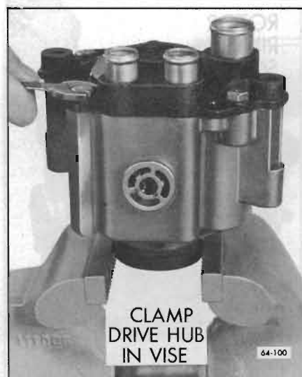
Figure 66-5—Air Pump Correctly Mounted for Disassembly
