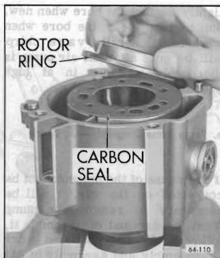
Figure 66-15—Installing Carbon Seal and Rotor Ring
