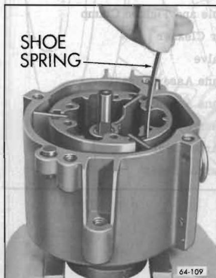
Figure 66-14—Installing Shoe Springs
