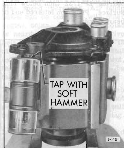
Figure 66-6—Removing Housing End Cover
