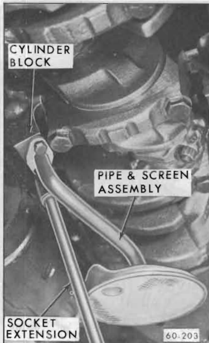
Figure 60-248—Installation of Pipe and Screen Assembly
