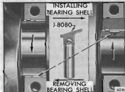
Figure 60-225—Removal and Installation of Crankshaft Bearing Upper Shell
