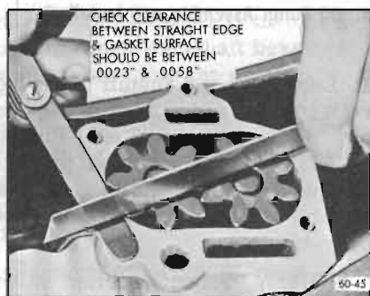
Figure 60-144—Checking Oil Pump Gear End Clearance
