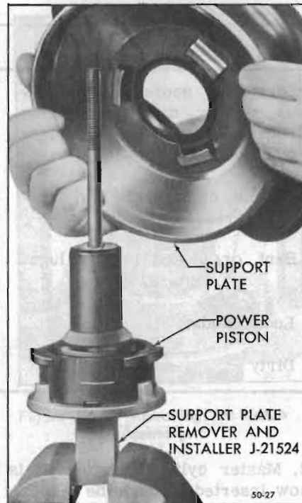
Figure 50-68—Installing Power Piston into Support Plate
