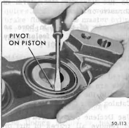
Figure 50-35—Removing Piston Boot
