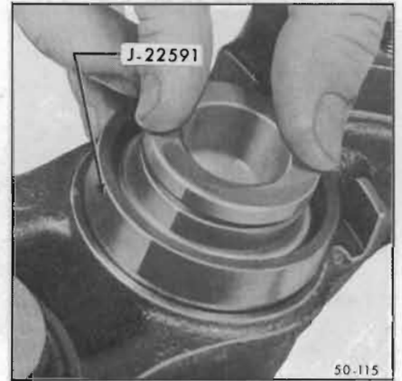
Figure 50-37—Installing Piston Assembly in Bore
