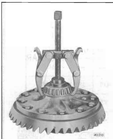
Figure 40-185—Removing Differential Side Bearing
