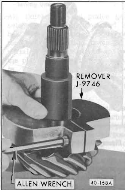
Figure 40-158—Installing Rear Pinion Bearing Remover
