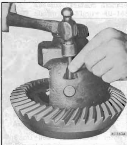
Figure 40-153—Removing Differential Pinion Axle Pin
