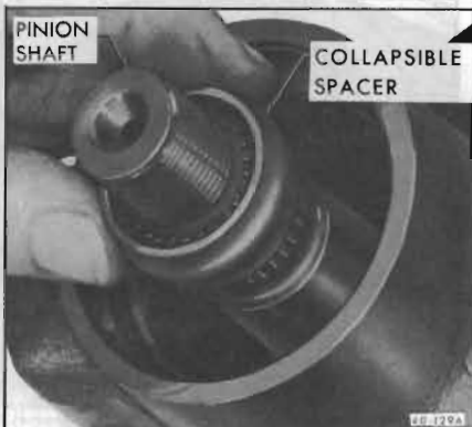
Figure 40-163—Installing Collapsible Spacer
