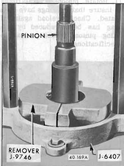
Figure 40-159—Removing Rear Pinion Bearing
