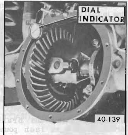
Figure 40-123—Checking Ring Gear to Pinion Backlash
