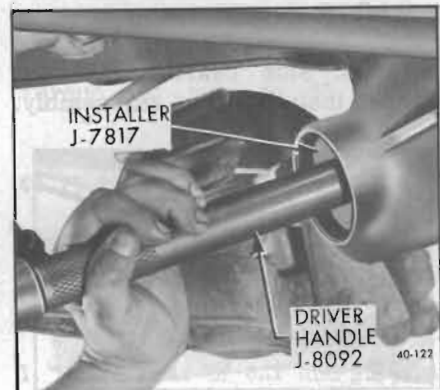
Figure 40-108—Installing Front Pinion Bearing Outer Race
