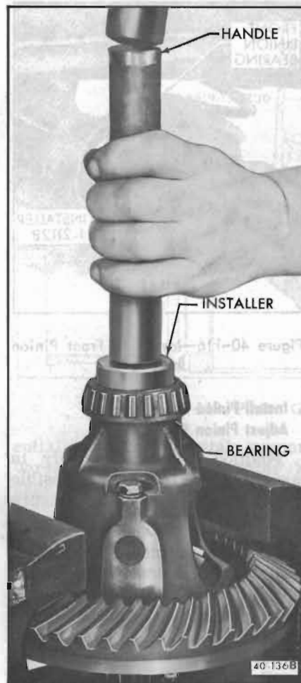
Figure 40-121—Installing Differential Side Bearings
