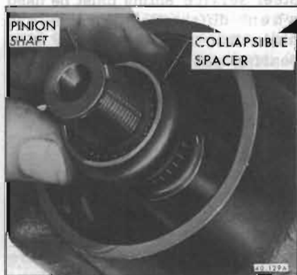
Figure 40-115—Installing Collapsible Spacer
