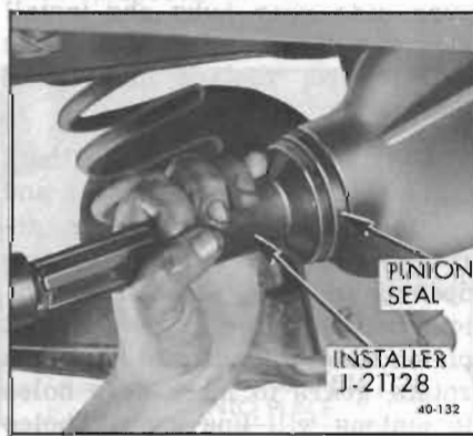
Figure 40-117—Installing Pinion Oil Seal
