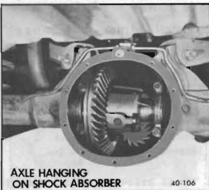
Figure 40-94—Differential Assembly in Position for Repair
