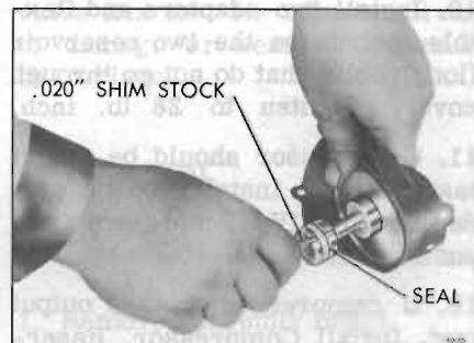
Figure 40-37—Installing Piston Seal
