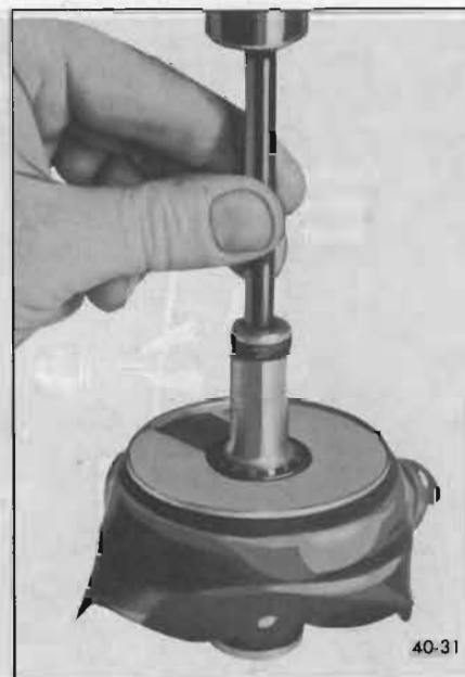
Figure 40-32—Installing Check Valve
