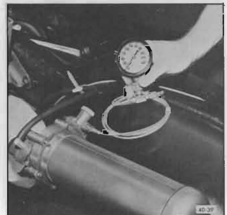
Figure 40-39—Test Gage Installed on Regulator Valve
