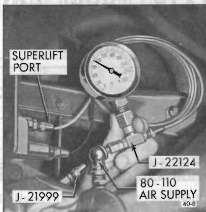
Figure 40-9—Connect Test Gage to Superlift Outlet
