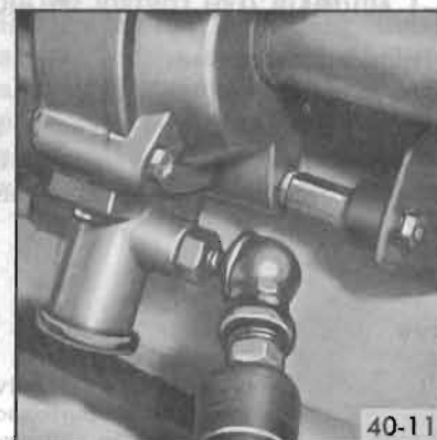
Figure 40-12—Filling System Through Service Valve
