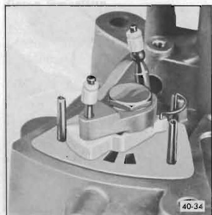
Figure 40-35—Installing Distributor Arm Assembly
