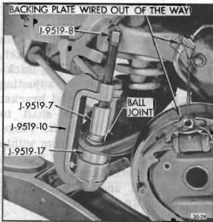
Figure 30-32—Lower Ball Joint Remover in Place
