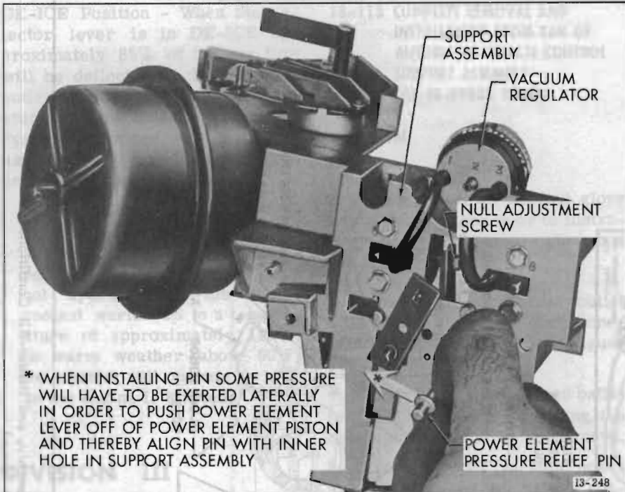
Figure 13-205—Installing Pressure Relief Pin into Support Assembly (45-46-48000 Series)
