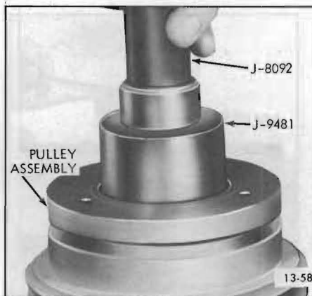
Figure 13-58—Installing Pulley Assembly
