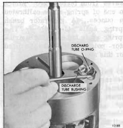
Figure 13-88—Installing Discharge Tube "O" Ring and Bushing
