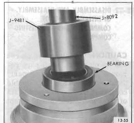
Figure 13-55—Installing Bearing into Pulley Assembly
