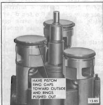
Figure 13-85—Pistons Position in "Stair-Step" Arrangement
