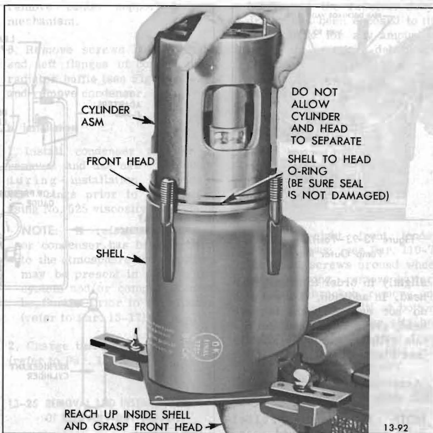
Figure 13-92—Installing Cylinder Assembly and Front Head in Shell
