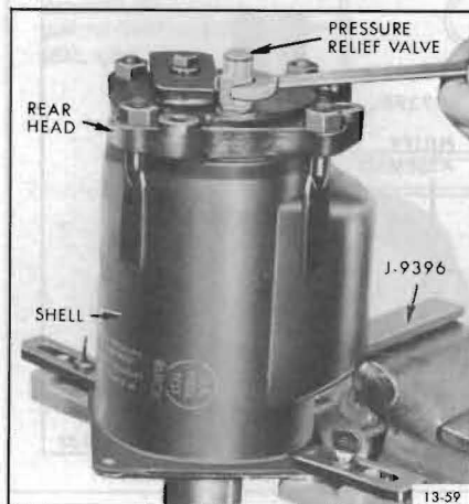
Figure 13-59—Compressor Installed in Holding Fixture
