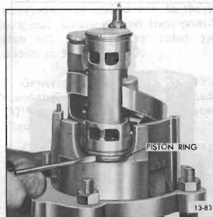
Figure 13-83—Compressing Front Piston Rings
