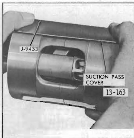
Figure 13-86—Installing Suction Pass Cover
