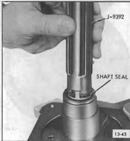
Figure 13-43—Removing or Installing Shaft Seal
