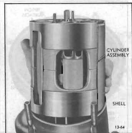
Figure 13-64—Removing Cylinder Assembly
