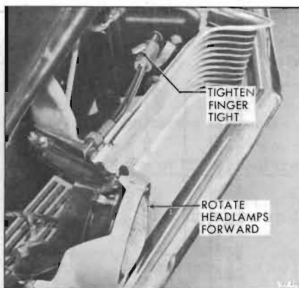
Figure 120-43—Locking Headlamps in Forward Position
