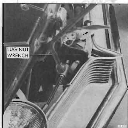
Figure 120-42—Loosening Set Screws
