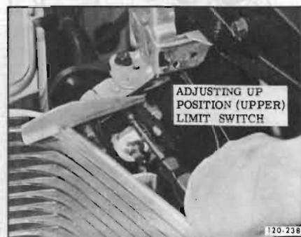
Figure 120-50—Adjusting Up Position Limit Switch
