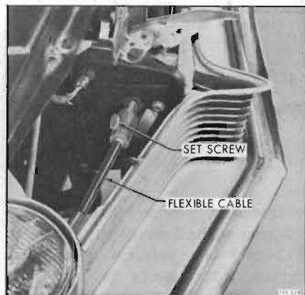
Figure 120-41—Locating Flexible Cable Set Screws
