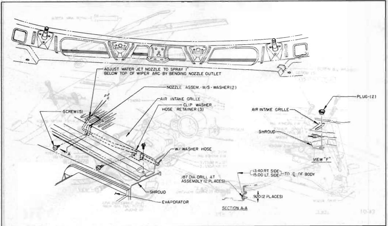
Figure 10-39—Washer Nozzle Aiming - 45-46-48000 Series
