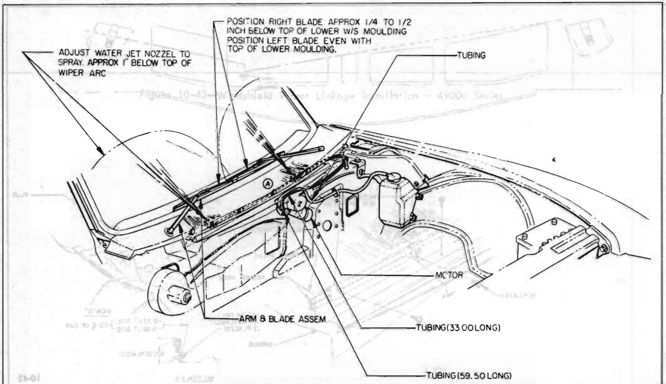
Figure 10-40—Windshield Wiper and Washer Installation - 49000 Series
