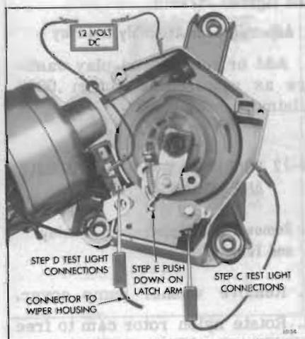
Figure 10-35—Test Light Checks
