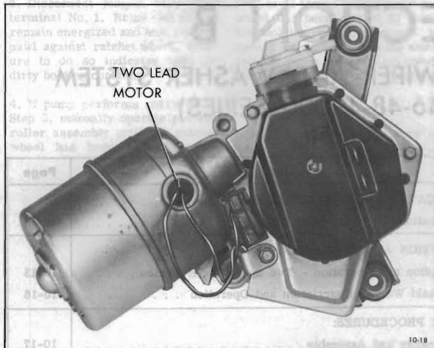
Figure 10-18—Windshield Wiper Motor - Two Speed
