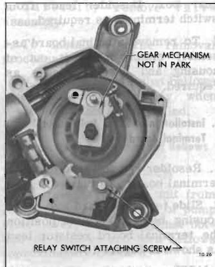
Figure 10-26—Removing Relay Switch Assembly
