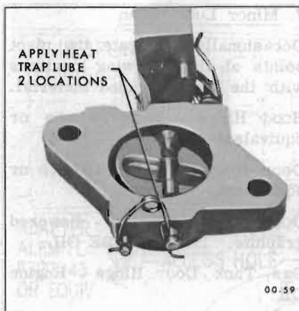
Figure 00-11—Lubricating Points on Manifold Heat Control Valve - 225, 300 and 340 Cu. In. Engine
