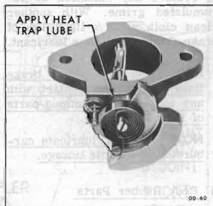
Figure 00-12—Lubricating Points on Manifold Heat Control Valve - 400 and 430 Cu. In. Engine
