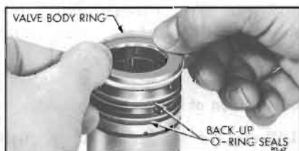
Figure 90-47—Installing Valve Body Rings
