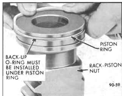
Figure 90-59—Installing Rack-Piston Ring on Rack-Piston Nut
