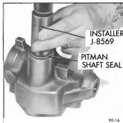
Figure 90-16—Installing Pitman Shaft Seal
