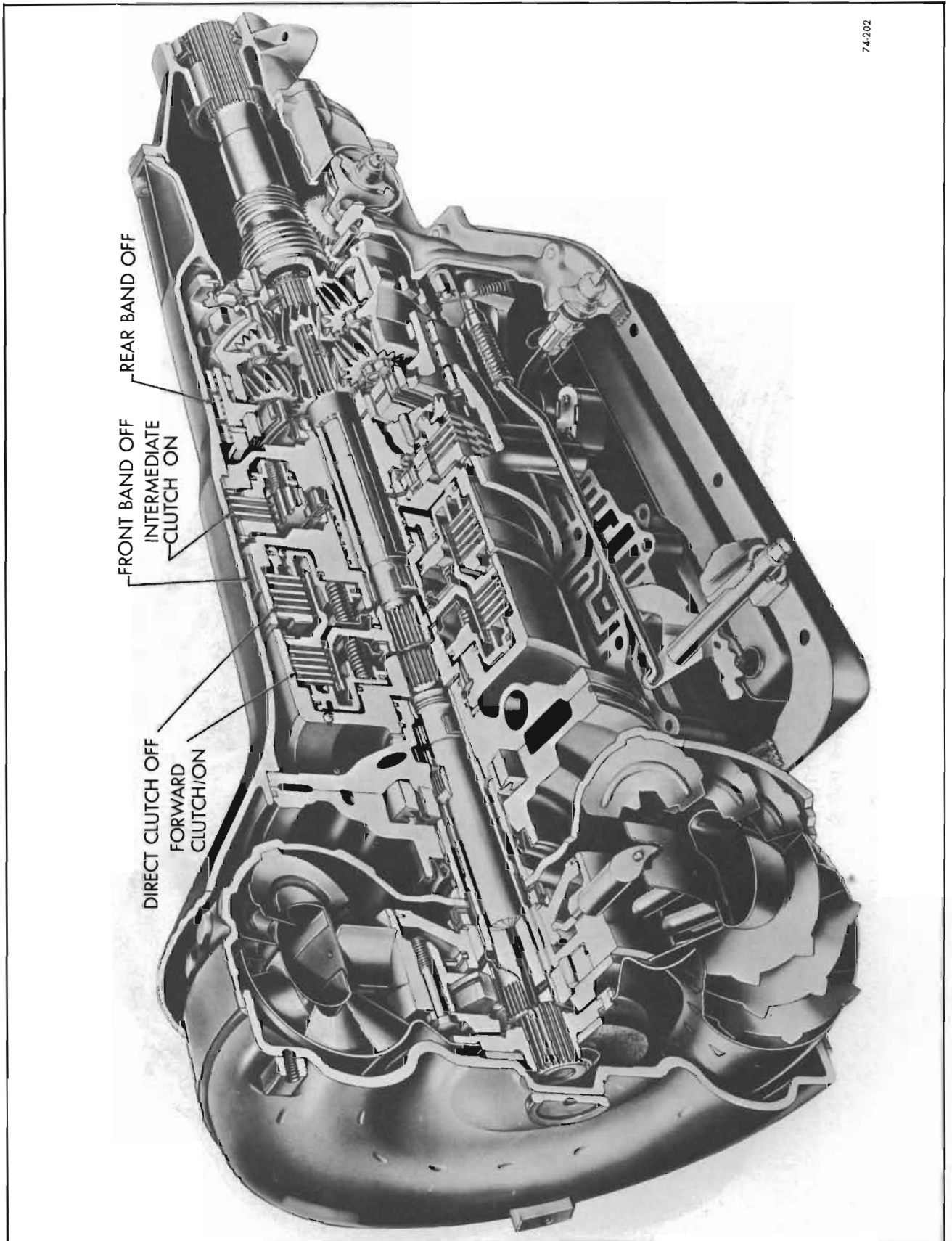
Figure 74-202—Drive Range - Second Gear
