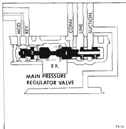
Figure 74-16—Pressure Regulator Valve (First Stage Regulation)
