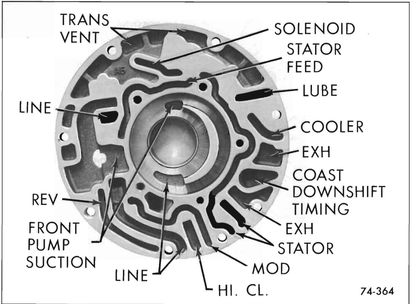
Figure 74-364—Oil Passages in Pump Body
