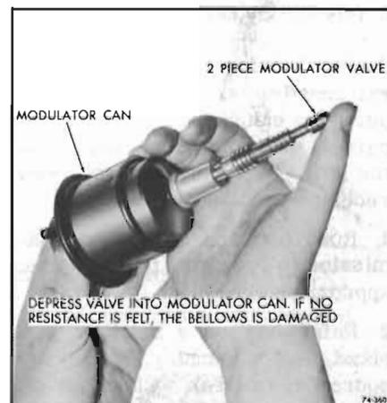
Figure 74-360—Checking Modulator Can Assembly
