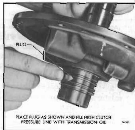
Figure 74-361—Checking Cross Leakage Between Pump Cover and Stator Shaft
