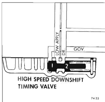
Figure 74-33—High Speed Down Shift Timing Valve Regulated
