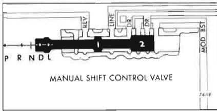
Figure 74-18—Manual Shift Control Valve
