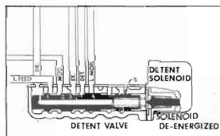
Figure 74-31—Solenoid Valve De-Energized
