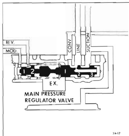
Figure 74-17—Pressure Regulator Valve (Second Stage Regulation)
