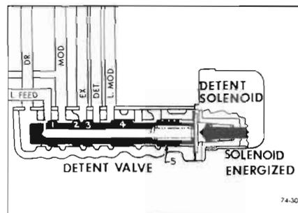
Figure 74-30—Solenoid Valve Energized
