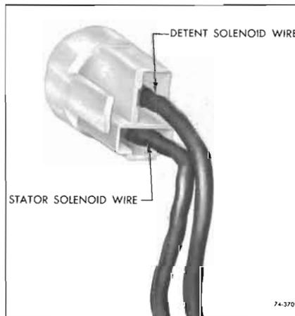
Figure 74-370—Location of Solenoid Wires
