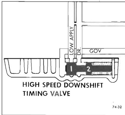
Figure 74-32—High Speed Down Shift Timing Valve
