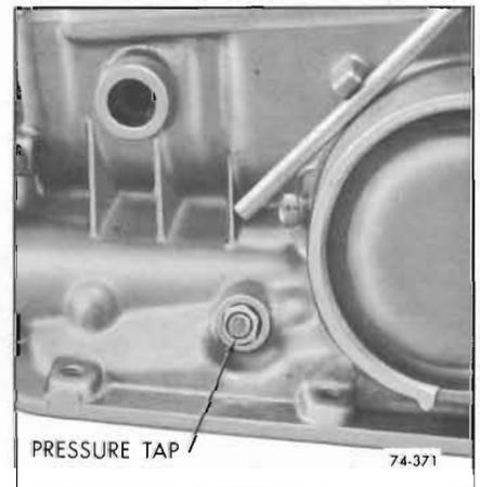
Figure 74-371— Super Turbine "300" Transmission Pressure Checks
