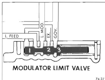
Figure 74-27—Modulator Limit Valve (First Stage)
