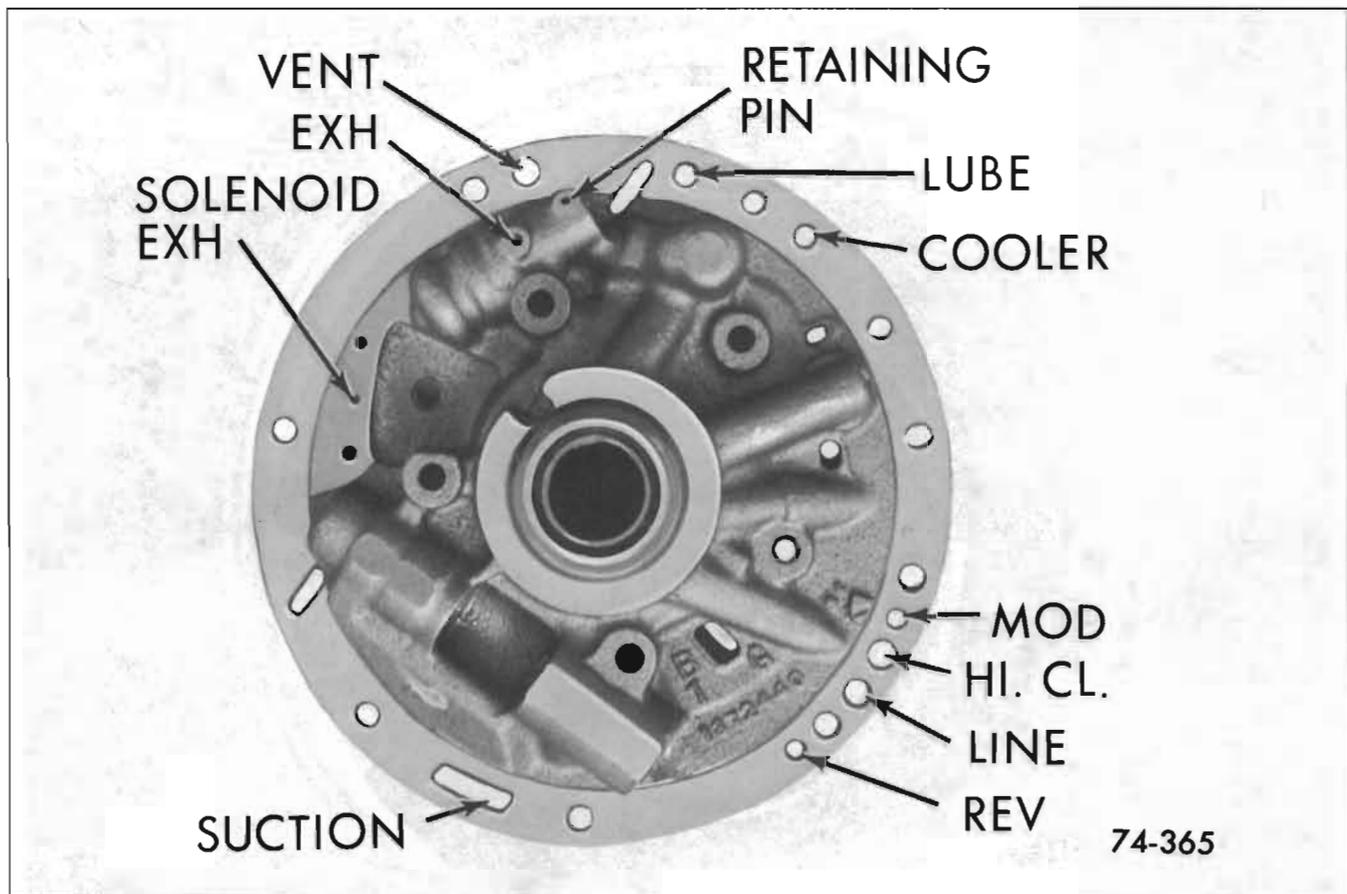
Figure 74-365—Oil Passages in Rear Face of Pump Cover
