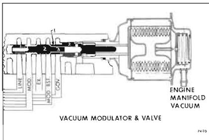
Figure 74-25—Vacuum Modulator and Valve
