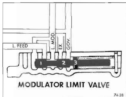
Figure 74-28—Modulator Limit Valve (Second Stage)
