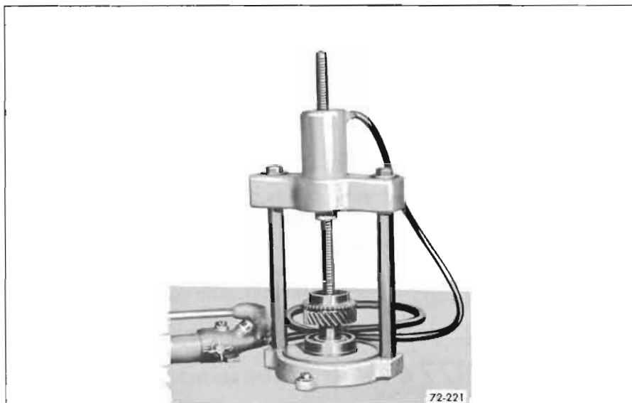
Figure 72-221—Installing Main Drive Gear Bearing
