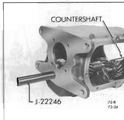
Figure 72-8—Removing Countershaft
