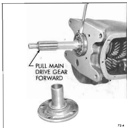
Figure 72-4—Removing Front Main Bearing
