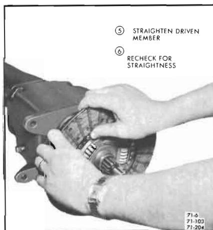
Figure 71-6—Checking Driven Plate Run-out
