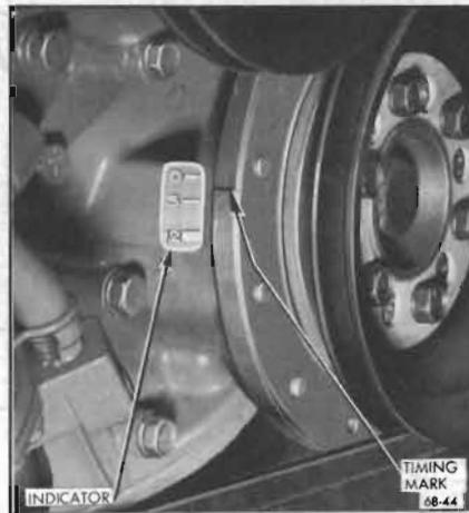
Figure 68-44—Ignition Timing Mark and Indicator - 400, 401 and 425 Engines
