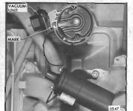
Figure 68-47—Installing Distributor in 400, 401 and 425 Engines
