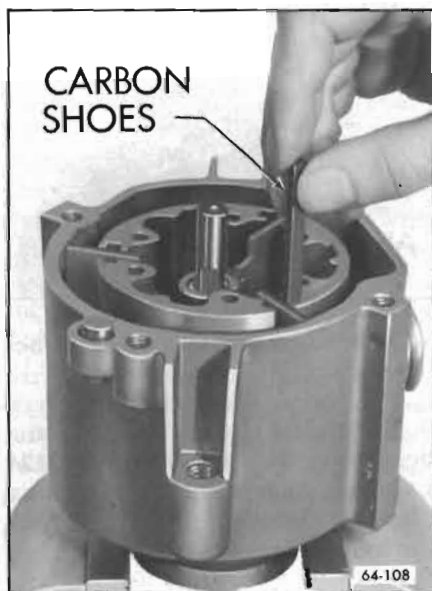
Figure 64-108—Installing Carbon Shoes
