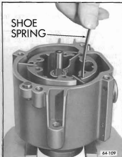
Figure 64-109—Installing Shoe Springs
