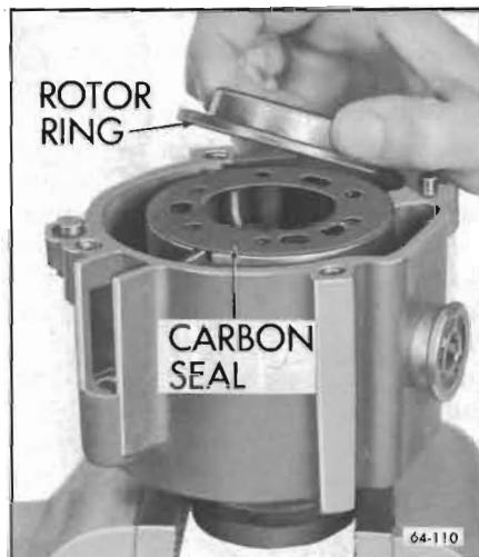
Figure 64-110—Installing Carbon Seal and Rotor Ring
