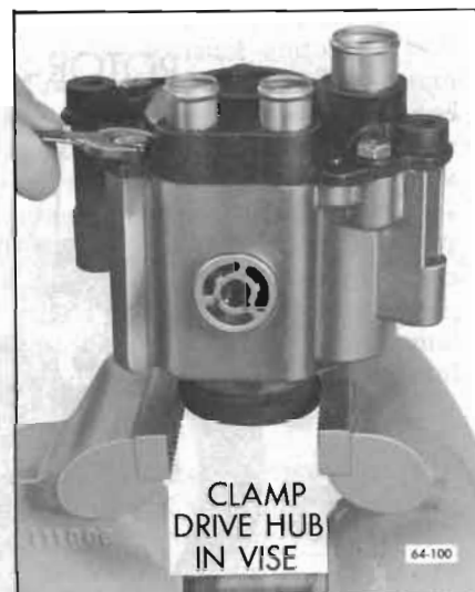
Figure 64-100—Air Pump Correctly Mounted for Disassembly
