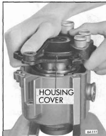
Figure 64-111—Installing Housing Cover
