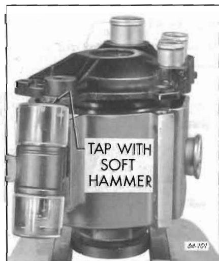
Figure 64-101—Removing Housing End Cover
