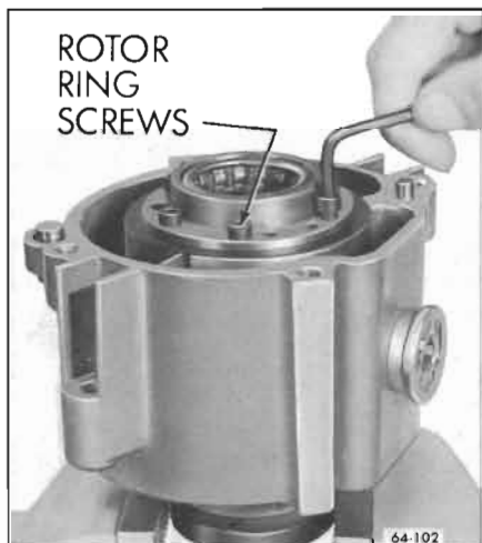
Figure 64-102—Removing Rotor Ring Screws
