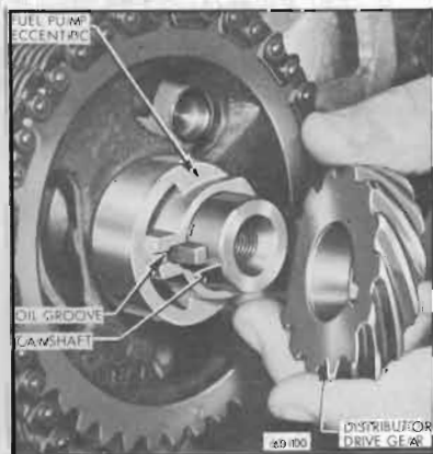
Figure 60-100—Fuel Pump and Distributor Drive Gear Installation
