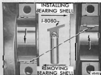
Figure 60-85—Removal and Installation of Crankshaft Bearing Upper Shell
