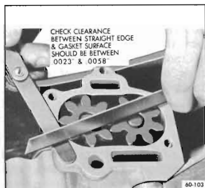
Figure 60-103—Checking Oil Pump End Clearance
