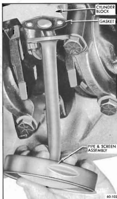
Figure 60-102—Installation of Pipe and Screen Assembly
