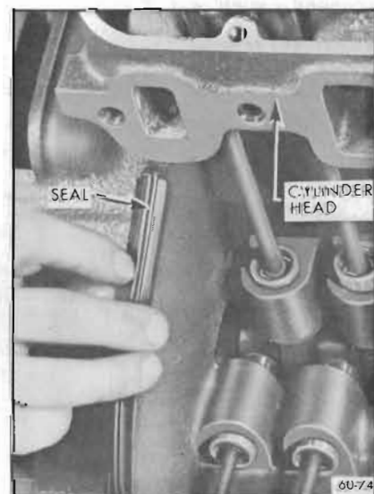
Figure 60-74—Installation of Intake Manifold Gasket Seal
