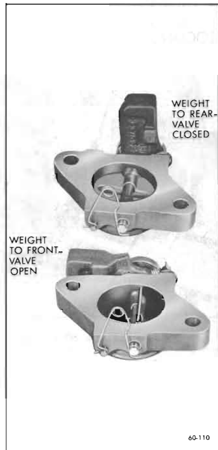
Figure 60-110—Manifold Heat Control Valve
