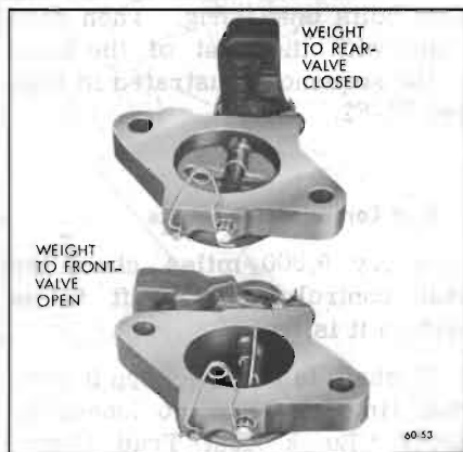
Figure 60-53—Manifold Heat Control Valve
