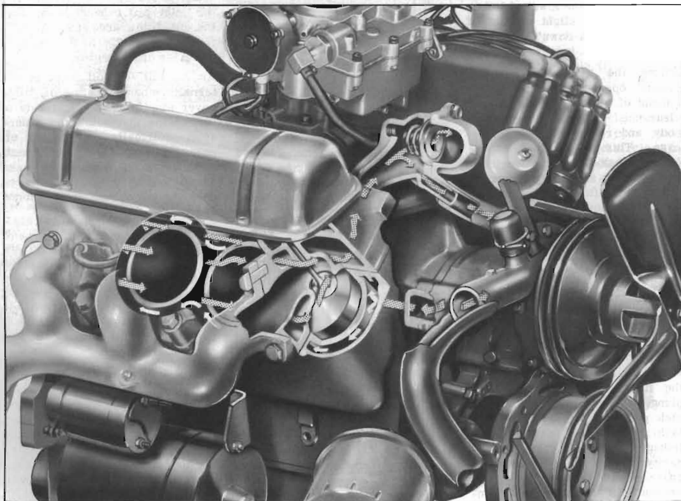
Figure 60-9—V-6 Cooling System
