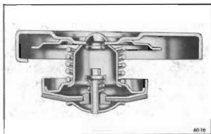
Figure 60-10—Radiator Pressure Cap Cross Section
