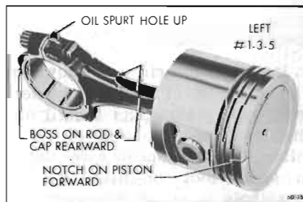
Figure 60-36—Left Piston and Rod Assembly
