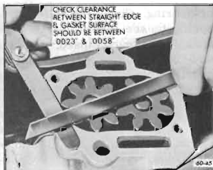
Figure 60-45—Checking Oil Pump Gear End Clearance
