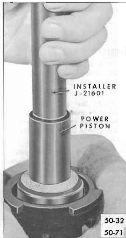
Figure 50-71—Installing Floating Control Valve Assembly
