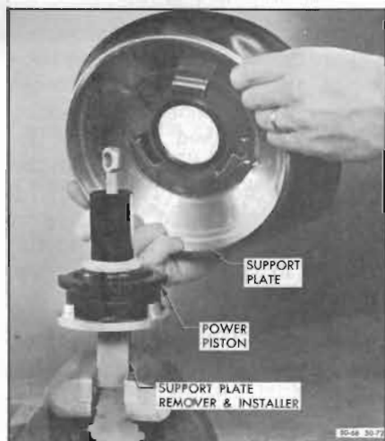
Figure 50-72—Installing Power Piston Into Support Plate
