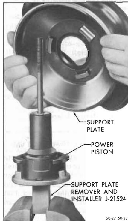
Figure 50-33—Installing Power Piston into Support Plate
