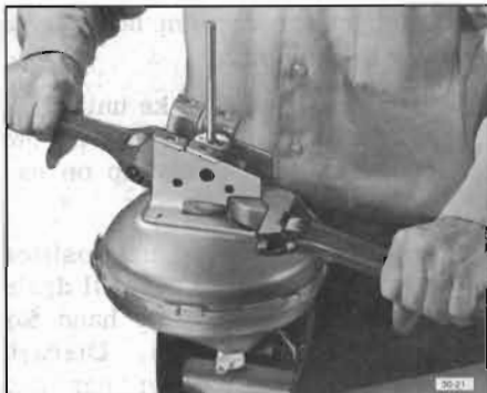
Figure 50-21—Power Brake Unit Positioned in a Vise
