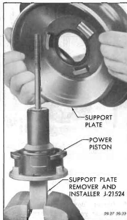
Figure 50-27—Removing Support Plate
