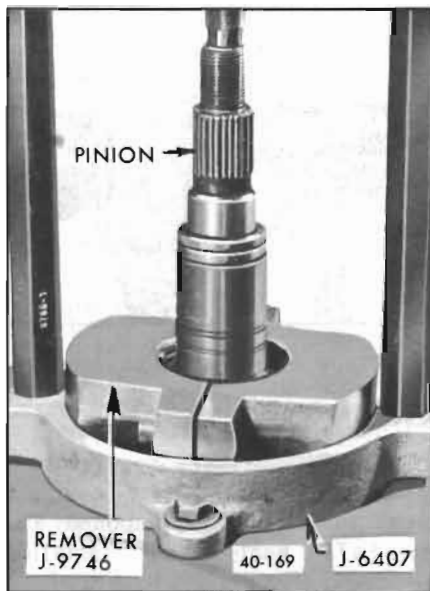
Figure 40-169—Removing Rear Pinion Bearing
