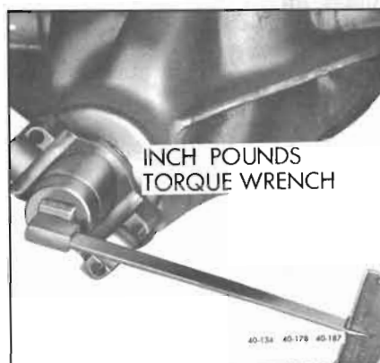
Figure 40-187—Checking Differential Case Preload
