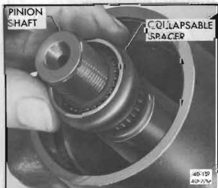
Figure 40-174—Installing Collapsible Spacer
