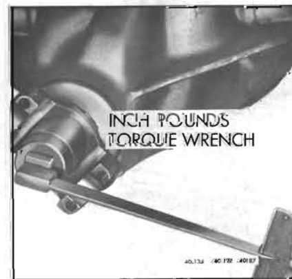
Figure 40-178—Checking Pinion Bearing Preload
