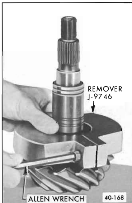
Figure 40-168—Installing Rear Pinion Bearing Remover
