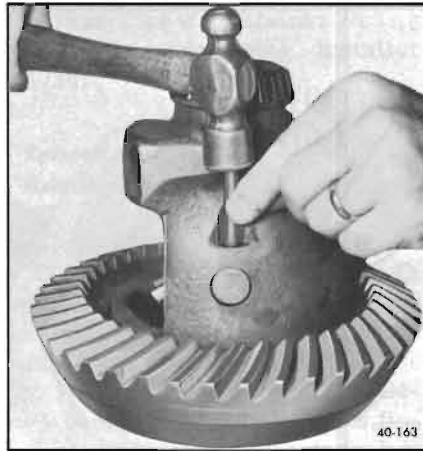
Figure 40-163—Removing Differential Pinion Axle Pin
