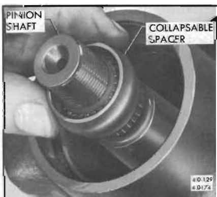
Figure 40-129—Installing Collapsible Spacer
