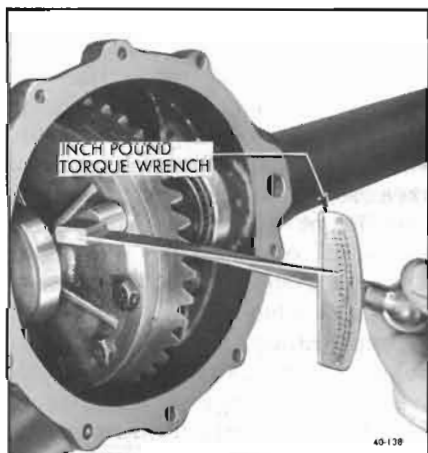
Figure 40-138—Checking Differential Case Preload
