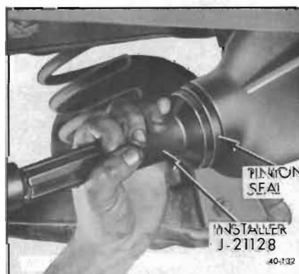
Figure 40-132—Installing Pinion Oil Seal
