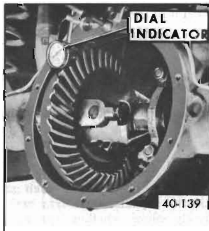
Figure 40-139—Checking Ring Gear To Pinion Backlash
