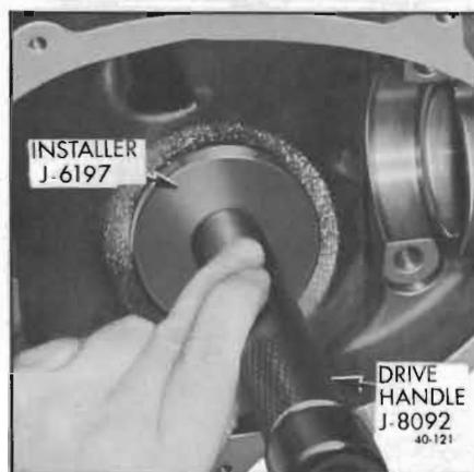
Figure 40-121—Installing Rear Pinion Bearing Outer Race
