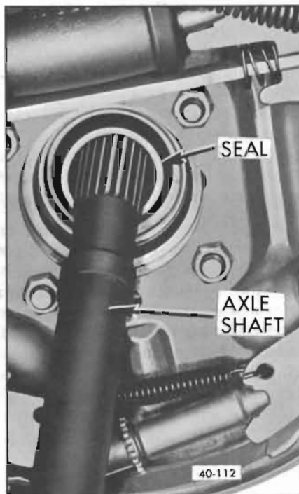
Figure 40-112—Removing Axle Shaft Seal
