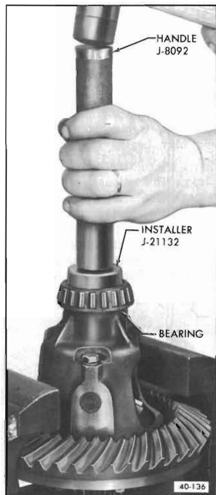
Figure 40-136—Installing Differential Side Bearings
