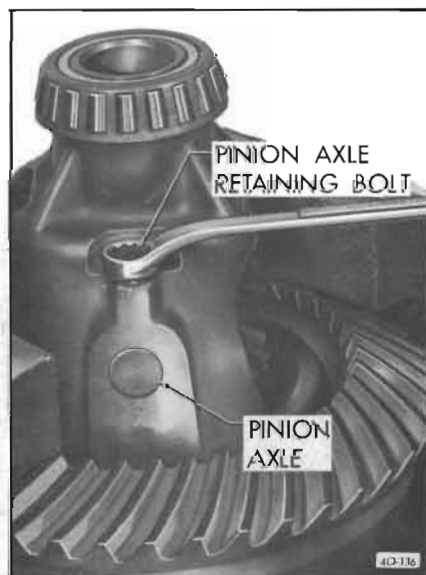
Figure 40-116—Removing Pinion Axle Retaining Bolt
