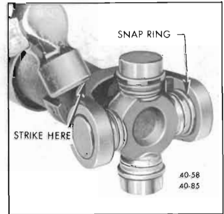
Figure 40-85—Seating U-Joint Snap Rings
