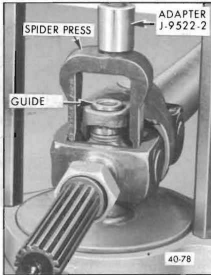
Figure 40-78—Removing Bearing With Guide and Spacer in Place
