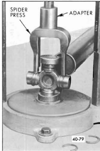
Figure 40-79—Pressing Out U-Joint Bearing
