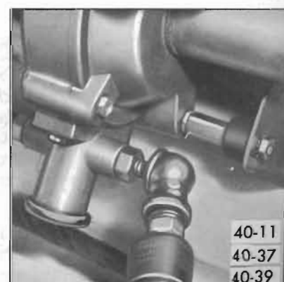
Figure 40-11—Filling System Through Service Valve
