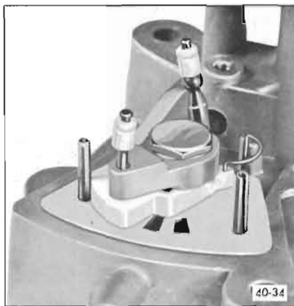
Figure 40-34—Installing Distributor Arm Assembly
