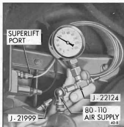
Figure 40-8—Connect Test Gage to Superlift Outlet
