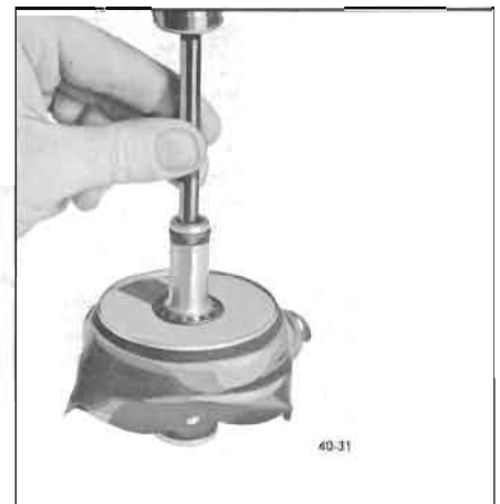
Figure 40-31—Installing Check Valve
