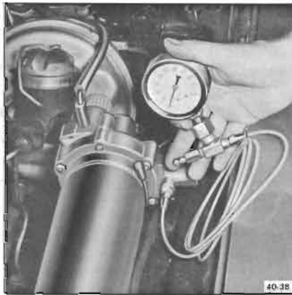
Figure 40-38—Test Gage Installed on Regulator Valve
