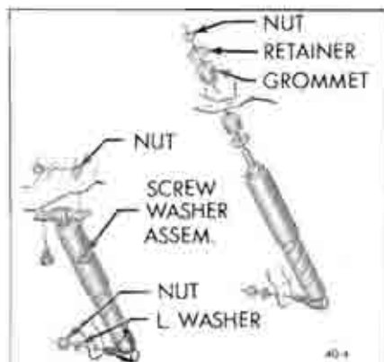
Figure 40-4—Rear Shock Absorber Installation
