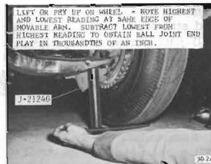
Figure 30-24—Ball Joint Checking Gauge Installed
