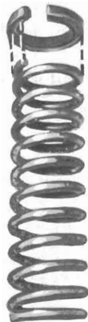
Figure 30-19—Installing Shim On Spring
