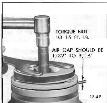
Figure 13-49—Torquing Shaft Nut
