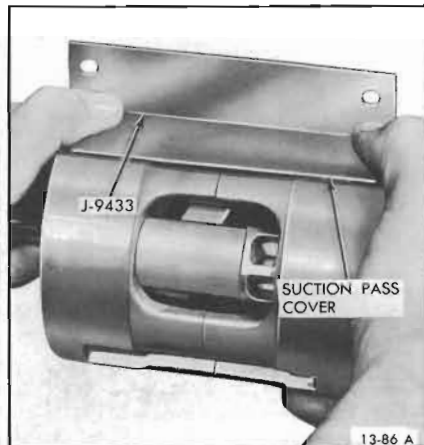
Figure 13-86—Installing Suction Pass Cover and Seal
