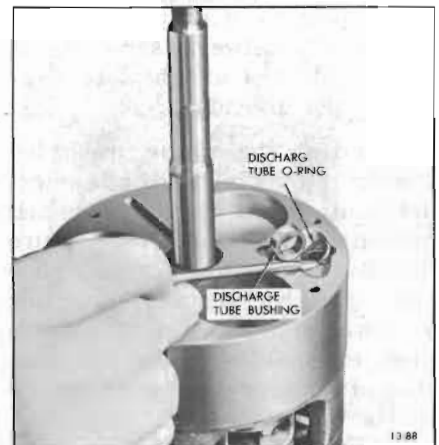
Figure 13-88—Installing Discharge Tube O-Ring and Bushing
