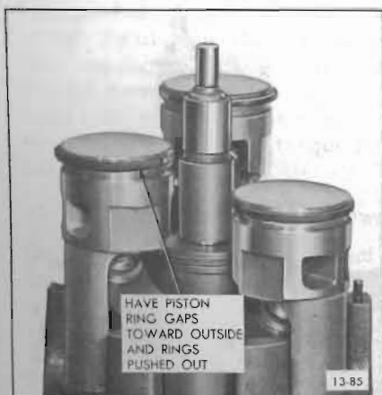
Figure 13-85—Pistons Position in “Stair-Step” Arrangement
