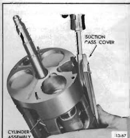
Figure 13-67—Removing Suction Pass Cover and Seal
