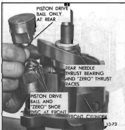
Figure 13-73—Installing Piston into Cylinder Half
