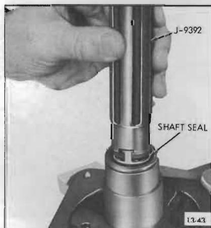
Figure 13-43—Removing or Installing Shaft Seal
