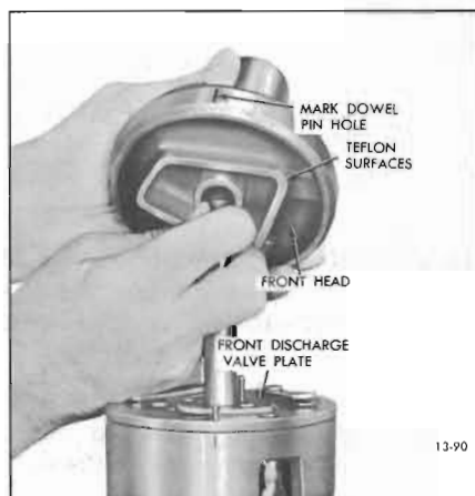
Figure 13-90—Placing Front Head on Cylinder Assembly
