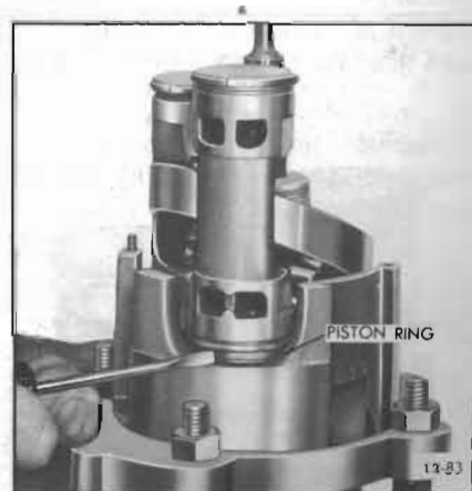
Figure 13-83—Compressing Front Piston Rings
