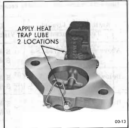
Figure 00-13—Lubricating Points on Manifold Heat Control Valve
