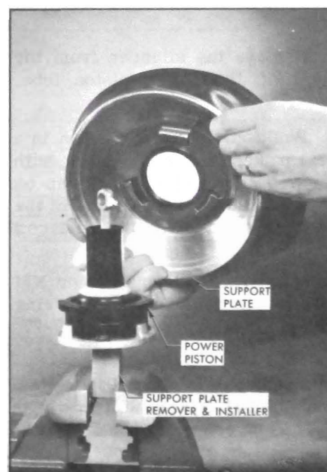
Figure 9-26—Removing Support Plate
