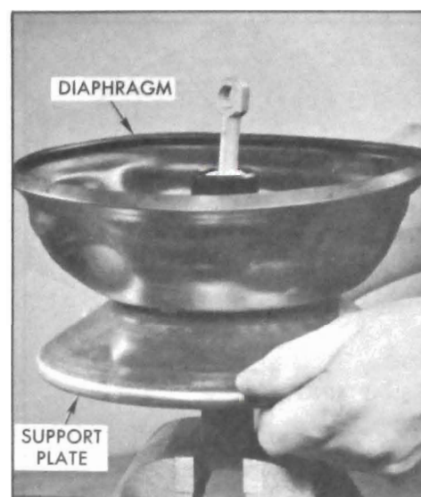
Figure 9-25—Positioning Power Piston on Support Plate Remover
