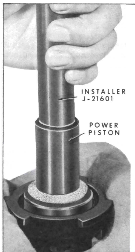
Figure 9-30—Seating Floating Control Valve Assembly
